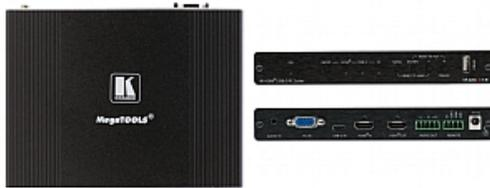
VP-426C is a high-performance digital scaler for HDMI, USB Type-C and computer graphics signals. The unit up- or down-scales the selected video signal to resolutions up to 4K@60 (4:4:4) at a maximum data rate of 18Gbps (6Gbps per graphic channel). The user selects the HDMI, USB Type-C, or VGA input and the scaled output is sent to the HDMI output
